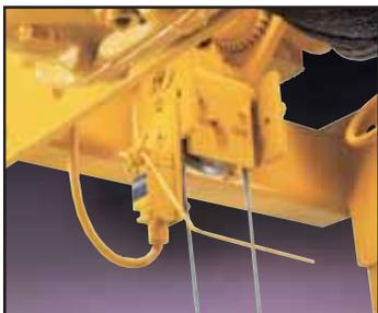
**Upper Block-Operated Limit Switch (Except Winches)**
